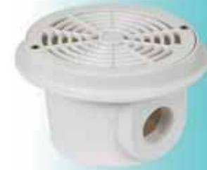
**Squared Main Drain.** Made of white ABS plastic. Grille fixed w/stainless steel screws, Ø50 mm female slip blind connection at the bottom for hydrostatic valve connection.
