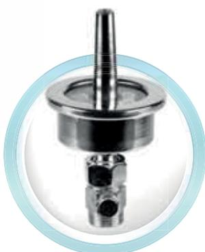
“**SPOT 06-K**” Underwater light coupled with Finger fountain nozzle. 304 quality stainless steel body and single union. Nozzle (Ø10 mm) bottom connection is with swivel system and regulation valve (1”). 15° light angle with Power LED. 13 different light models are available and are controlled by a Central Control Panel. With 1 m Cable.
