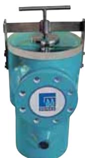
Fiberglass reinforced polyester pre-filter. Loose flange connection and 20 l capacity. Pipe connections can be produced according to demand. The basket and opening mechanism are made of stainless steel. Transparent acrylic lid. Can be used up to 160 mm connections.
