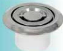
**Stainless Steel Wall Inlet for Concrete Pools.** Body is injected of white ABS plastic dressed with AISI 304 quality stainless steel plate. The butterfly of nozzle is made of solid inox inlets stainless steel and the sphere is of acrylic transparent plastic with adjustable ball for alternative discharges.
