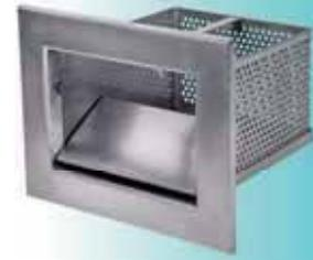
**Stainless Steel Level Adjustable Lid for Concrete Pools.** Made of AISI 304 Stainless steel Dimensions:180 x 180 mm. Height level can be adjustable from 60 to 110 mm.
