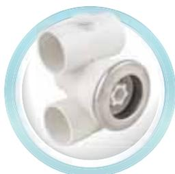
**"SP-1434ASS" Model Massage Jet.** Water and air connection Ø 50, PVC, 2" inlet included. Frame is stainless steel. Recommended flow; 1,5 m<sup>3</sup>/h - 7 mwh
