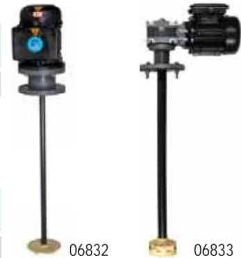
Motorized Slow Mixer. Made of PVC plastic. 70 rpm speed slow mixer. 0.13 KW / 220 V / 50 Hz. Shaft length: 600 mm.
