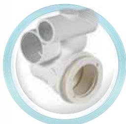
**"Magna" Model Massage Jet Body.** Water connection d.50, air connection d.32, excluding nozzle. Recommended flow; 2,7 m<sup>3</sup>/h - 7 mwh
