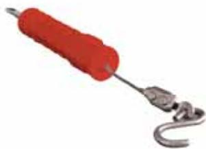
**Ergonomic Separator Tensioner.** Body made of GF-PP and accessories from AISI 316. complete with 7 mm thick hook, SS rope fixing accessories. Threaded tension rod and easy grip plastic body allows easy tightening up to 130 mm. Can only used with SS lane ropes
