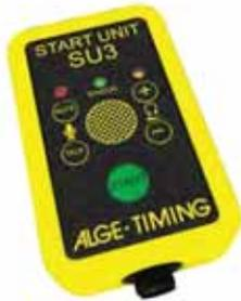
**Start Unit:** Complete with integrated microphone and start button.
