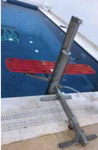
**Pool lift for disabilities:** Hydraulic lift made of AISI 304 stainless steel. Garden irrigation hose has to be connected to a hydraulic lift. Required minimum water pressure is 3,5 kg/cm<sup>2</sup>. User friendly installation and can easily be adapted to an existing pool.
