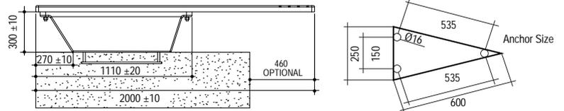
**CLASSIC 200 HR DIVING BOARD** Base and board made in laminated polyester and fiberglass. Complete with stainless steel handrails.
