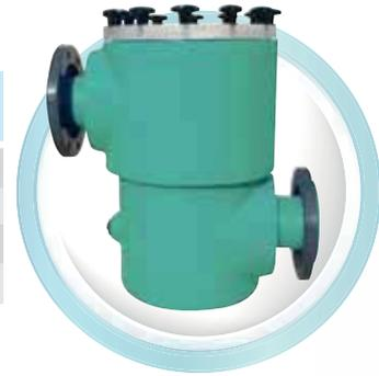
Fiber glass reinforced polyester pre-filter. Loose flange connection. Ø280, Ø315 and Ø355 has **125 l** Ø400 and Ø450 has **285 l** capacity. AISI 304 quality stainless steel basket. Transparent acrylic lid. Can be used up to 225 mm connections.
