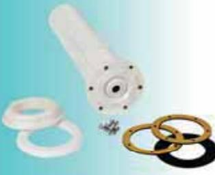
**Wall Conduit-Inlet for Liner Pools.** Specially designed for concrete-shell liner pools. Injected of white ABS plastic with adjustable ball for alternative discharges. Complete with flange, gaskets, stainless steel screws, front cover and back locking nut. Flange connections can be with brass cavities or plastic nests.
