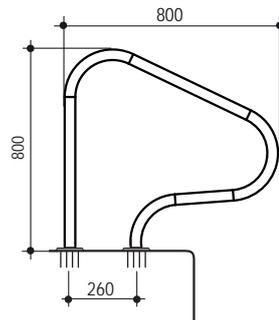
**Cross Grab Rail:** Ø42 mm. Made of Ø42 mm AISI 304 stainless steel pipe. Complete with monoblock rectangular fixing plate, bolts and bolt plugs.
