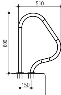
**Deep Grab Rail:** 800 x 800 mm. Made of Ø42 mm AISI 304 stainless steel pipe. Complete with fixing plates, bolts and bolt plugs.
