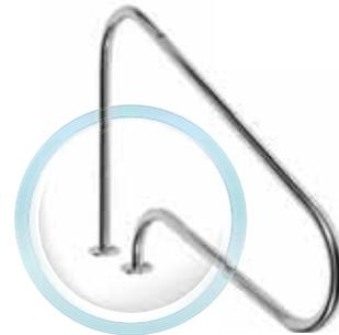
**LATERAL GRAB RAIL WITH FIXING PLATES.** Made of AISI 304 grade polished stainless steel Ø42 mm pipe. Complete with fixing plates and screws.
