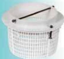
**Floor Inlet - Adjustable for Concrete Pools.** Injected of white ABS plastic, according to EU 13451-14.8.3" male threaded, Ø50 mm internal slip connection. Discharge can be regulated by means of an inner lid which can be screwed up and down.
