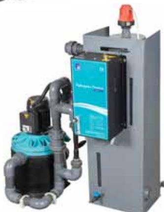
**GEMAS HYDROZONE Corona Discharge Compact Ozone Systems.** 5 g/h capacity, complete with jet pump, automatic gas discharge valve, PVC contact tank, deoxygenation active carbon tank, injector, PVC water trap tank, PVC base and column. Complete with necessary mechanical and electrical installation. It can be use with oxygen concentrator.
