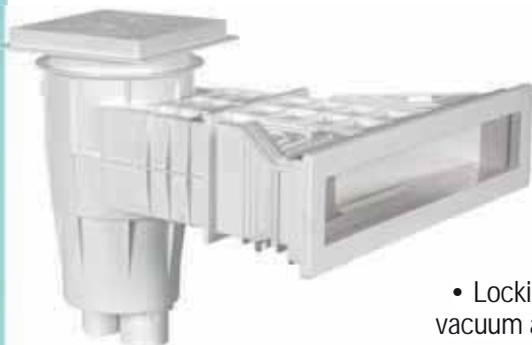
All Lux-Skimmer models are made of ABS plastic and equipped with "suction regulator" and locking mechanism of baskets against back pressure. Skimming by "buoy float" or "floating weir". Suction port: 2" female threaded. Second port: 1,5" female threaded supplied with blind cap. Overflow drainage: Ø40 mm female slip.
