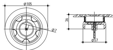
**Overflow Gutter Drain for Concrete Pools.** Made of white ABS plastic. 2½" male - threaded, Ø63 mm inside. Stainless steel screws included.
