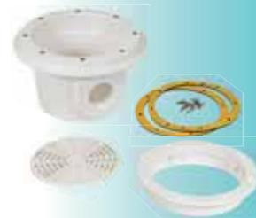
**Circular Main Drain with St. Steel Grille for Concrete Pools.** Body made of ABS plastic. Stainless steel grille fixed w/st. steel screws, Ø50 mm female slip blind connection at the bottom for hydrostatic valve connection.
