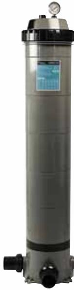
**GEMAS CARTRIDGE FILTER.** Body made in ABS plastic. Complete with manometer and air purge connections 1,5" BSP threaded. Max. operation pressure: 2.5 Bar.
