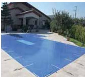
**Pool Cover.** Made of PVC. Peripheral reinforcement of 5 cm. Laterals at each 1 m of the periphery are used to stretch the cover over pool surface by means of stainless steel springs attached to special bronze retractable anchors. Drain holes are available at the center to discharge the rain water. Complete with springs and retractable anchors.
