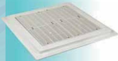
**Squared Grilles for Main Drain for Concrete Pools.** Fiberglass reinforced polyester frame with ext. dimensions of 60 x 60 cm complete with fixing screws. Max. recommended drain pipe size : Ø225 mm.
