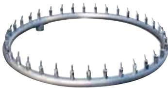
Plastic Water Star. Made of 36 pieces of 3/8" plastic finger jets. Dia Ø1000 mm, water jet Ø4,0 mm, connection 1,5".
