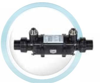
Heat Exchangers, Shell and Tube Type. With plastic body, AISI 316/Titanium-Corrugated Metal Coil. The plastic body is resistant to high pressure and corrosion. It is attractive in terms of cost advantage and quality. It works with hot water (90/70°C) from the boiler. Max. pressure: Primary (boiler side) circuit 6 bar, secondary (poolside) 2 bar. Connection fittings are ABS, O-rings are silicone.
