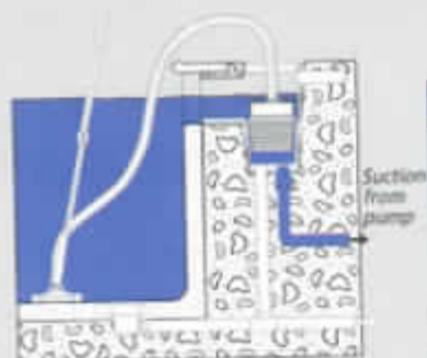
1- Suction connection for pool cleaner
