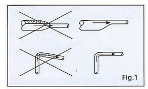
The pipes should be fitted in such a way that any pressure varioation caused by temperature changes do not effect the pump. If the piping is very long and/or high support the pump in front and behind. It is reccomendable to put a retention or check valve at the outlet.
