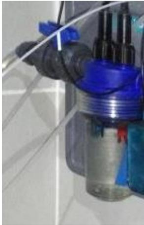
The water from the suction collector is connected to the flow cell to be measured.
