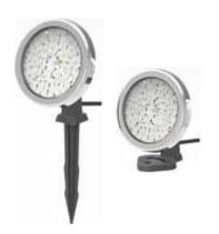
**Product Details:** Designed for fountains and landscape lighting. It has a stainless steel frame. With 72 SMD LED. Complete with polycarbonate light body, epoxy PCB and 1.0 m long 2 x 0.75 cable and mounting leg/stake. 120°- IP68. The pedestal light can be used as a replacement light for LED conversion in all commercially available PAR38 light products. The product is patented.
