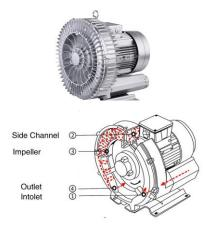
**Product Details:** The impellers are mounted directly on the motor shaft for noncontact compression entirely without friction. Maximum operational reliability, even at high differential is ensured by the arrangement of the bearings outside the compression chamber.
