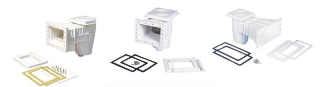
**Product Details:** All skimmer models are made in ABS plastic and equipped with "suction regulator" and locking mechanism of baskets against back pressure. Skimming by **"buoy float"** or **floating weir"**. Suction port: 1 1/2" female threaded (2" also possible upon request), Ø 63 mm external slip. Second port: Ø 50 mm female slip. Overflow drainage: Ø 40 mm female slip.
