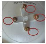
Cables should be connected according to sign on the bulbs as shown on the right picture.
