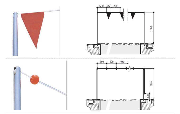
**PS:** Designed to be fixed with "14410" or "14420" anchors which are not included. Two sets are necessary for a competition pool.
